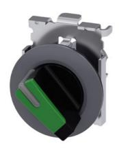
Selector switch, illuminable, 30 mm, round, Metal, matte, green, selector switch, short, front ring for flush installation, 2 switch positions O<I, momentary contact type, Actuating angle 45°, 10:30h/12h, with laser labeling, upper case
