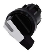
Selector switch, illuminable, 22 mm, round, plastic, white, selector switch, long, 2 switch positions O-l, latching, actuating angle 90°, 10:30h/13:30h, with laser labeling, upper case
