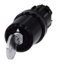
Key-operated switch BKS, 22 mm, round, plastic, lock number S1, with 2 keys, 3 switch positions I>O<II, momentary contact on the left, latching on the right, actuating angle  $2x45^{\circ}$ , 10:30h/12h/13:30h, key removal O, with laser labeling, lower case
