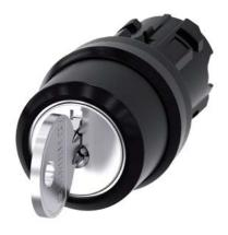
RONIS key-operated switch, 22 mm, round, plastic, special lock, with 2 keys, 3 switch positions I>O<II, momentary contact on the left, latching on the right, actuating angle  $2x45^{\circ}$ , 10:30h/12h/13:30h, Key removal II, possible special locks: SB31, 421, 455
