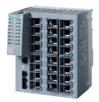
SCALANCE XC224 manageable Layer 2 IE switch; IEC 62443-4-2 certified; 24x 10/100 Mbit/s RJ45 ports; 1x console port, diagnostics LED; redundant power supply; temperature range -40 °C to +70 °C; assembly: DIN rail/S7 mounting rail/wall Office redundancy functions features (RSTP, VLAN,...); PROFINET IO device Ethernet/IP-compliant, C-plug slot;
