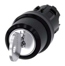
RONIS key-operated switch, 22 mm, round, plastic, lock number SB30, with 2 keys, 3 switch positions I-O-II, latching, actuating angle 2x45°, 10:30h/12h/13:30h, Key removal II, possible special locks: SB31, 421, 455 Z=50-unit packaging
