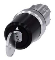
key-operated switch Siemens, 22 mm, round, metal, shiny, lock number SSG10, with 2 keys, 3 switch positions I-O-II, latching, actuating angle 2x45°, 10:30h/12h/13:30h, key removal I+O+II, Z=50-unit packaging
