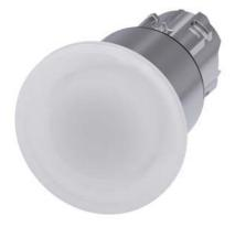
Illuminated mushroom pushbutton, 22 mm, round, metal, shiny, white, 40 mm, 3 switch positions, after pushing in Retraction to center position, after pulling out the button Retraction to center position, with laser labeling, inscription or symbol Customer-specific selection with SIRIUS ACT configurator (CIN)
