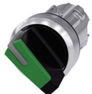
Selector switch, illuminable, 22 mm, round, metal, shiny, green, selector switch, short, 2 switch positions O-I, latching, actuating angle 90°, 10:30h/13:30h, Z=50-unit packaging
