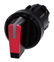
Selector switch, illuminable, 22 mm, round, plastic, red, selector switch, short, 3 switch positions I>O<II, momentary contact on the left, latching on the right, actuating angle 2x45°, 10:30h/12h/13:30h, with laser labeling, inscription or symbol Customer-specific selection with SIRIUS ACT configurator (CIN)
