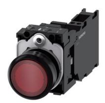
Illuminated pushbutton, 22 mm, round, plastic, red, pushbutton, flat, momentary contact type, with holder, 1 NO+1 NC, LED module with integrated LED 110 V AC, spring-type terminal, Z=20-unit packaging
