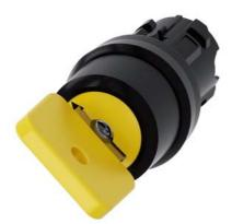
Key-operated switch O.M.R, 22 mm, round, plastic, lock number 73033, yellow, with 2 keys, 2 switch positions O<I, momentary contact type, Actuating angle 45°, 10:30h/12h, key removal O, with laser labeling, inscription or symbol Customer-specific selection with SIRIUS ACT configurator (CIN)
