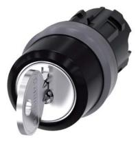
RONIS key-operated switch, 22 mm, round, plastic with metal front ring, special lock, with 2 keys, 3 switch positions I>O<II, momentary contact on the left, latching on the right, actuating angle 2x45°, 10:30h/12h/13:30h, key removal O, possible special locks: SB31, 421, 455
