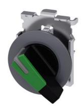
Selector switch, illuminable, 30 mm, round, Metal, matte, green, selector switch, long, front ring for flush installation, 2 switch positions O<I, momentary contact type, Actuating angle 45°, 10:30h/12h, with laser labeling, lower case
