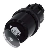
keyswitch BKS, 22 mm, round, plastic, special lock, with 2 keys, 2 switch positions O-I, latching, actuating angle 90°, 10:30h/13:30h, key removal I, note: for the BKS locking systems E1 - E25 supplied without key
