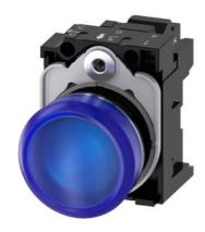
Indicator lights, 22 mm, round, metal, shiny, blue, lens, smooth, with holder, LED module with integrated LED 110 V AC, spring-type terminal, with laser labeling, upper case
