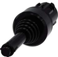
Coordinate switch, 22 mm, round, plastic, black, 4 switch positions, momentary contact type, with mechanical interlocking, with laser labeling, inscription or symbol Customer-specific selection with SIRIUS ACT configurator (CIN)
