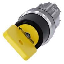
Key-operated switch O.M.R, 22 mm, round, metal, shiny, lock number 73033, yellow, with 2 keys, 2 switch positions O<I, momentary contact type, Actuating angle 45°, 10:30h/12h, key removal O, with laser labeling, upper case and lower case, always upper case at the beginning of the word
