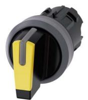
Selector switch, illuminable, 22 mm, round, plastic with metal front ring, yellow, selector switch, short, 3 switch positions I>O<II, momentary contact type, actuating angle 2x45°, 10:30h/12h/13:30h, with laser labeling, upper case and lower case, always upper case at the beginning of the word
