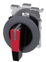
Selector switch, illuminable, 30 mm, round, Metal, matte, red, selector switch, long, front ring for flush installation, 3 switch positions I-O-II, latching, actuating angle  $2x45^{\circ}$ , 10:30h/12h/13:30h, with laser labeling, upper case and lower case, always upper case at the beginning of the word
