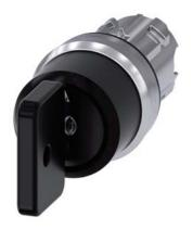
Key-operated switch O.M.R, 22 mm, round, metal, shiny, lock number 73034, black, with 2 keys, 3 switch positions I-O-II, latching, actuating angle 2x45°, 10:30h/12h/13:30h, Key removal I+O+II, with laser labeling, upper case
