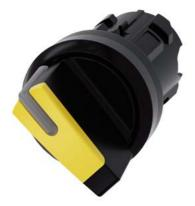
Selector switch, illuminable, 22 mm, round, plastic, yellow, selector switch, short, 2 switch positions O-I, latching, actuating angle 90°, 10:30h/13:30h, with laser labeling, upper case and lower case, always upper case at the beginning of the word
