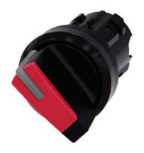
Selector switch, illuminable, 22 mm, round, plastic, red, selector switch, short, 2 switch positions O<I, momentary contact type, Actuating angle 45°, 10:30h/12h, with laser labeling, upper case and lower case, always upper case at beginning of line
