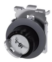
RONIS key-operated switch, 30 mm, round, Metal, matte, front ring for flush installation, lock number SB30, with 2 keys, 2 switch positions O-I, latching, actuating angle 90°, 10:30h/13:30h, key removal O+I, possible special locks: SB31, 421, 455, Z=50-unit packaging
