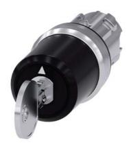
Key-operated switch BKS, 22 mm, round, metal, shiny, lock number S1, with 2 keys, 3 switch positions I-O<II, left latching, right momentary contact type, actuating angle  $2x45^{\circ}$ , 10:30h/12h/13:30h, key removal I, Z=50-unit packaging
