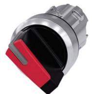
Selector switch, illuminable, 22 mm, round, metal, shiny, red, selector switch, short, 2 switch positions O<I, momentary contact type, Actuating angle 45°, 10:30h/12h, Z=50-unit packaging
