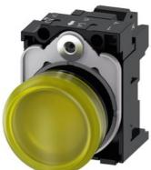
Indicator light, 22 mm, round, plastic, yellow, lens, smooth, with holder, LED module, with integrated LED 230 V AC, spring-type terminal, with laser labeling, upper case and lower case, always upper case at beginning of line
