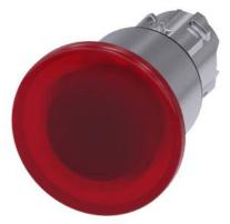
Illuminated mushroom pushbutton, 22 mm, round, metal, shiny, red, 40 mm, 3 switch positions, latches after pushing in, unlatches by pull-to-unlatch mechanism to center position, after pulling out the button Retraction to center position, with laser labeling, upper case and lower case, always upper case at the beginning of the word
