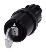
key-operated switch Siemens, 22 mm, round, plastic, lock number SSG10, with 2 keys, 3 switch positions I-O<II, left latching, momentary contact type on the right, actuating angle  $2\times45^\circ$ , 10:30h/12h/13:30h, key removal I, with laser labeling, upper case and lower case, always upper case at the beginning of the word
