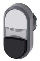
Illuminated twin pushbutton, 22 mm, round, plastic with metal front ring, white, black, pushbuttons, flat and raised, with laser labeling, upper case and lower case, always upper case at the beginning of the word
