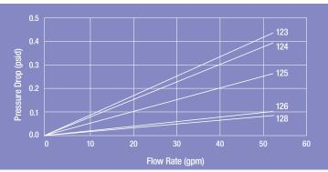
**Pressure Drop:** The Series 100 High Performance Filter Bags have low initial pressure drop ( $\Delta p$ ) in water as the chart indicates. The chart includes the pressure drop of a typical single vessel to assist you in sizing your filter system.
