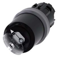
Key-operated switch IKON, 22 mm, round, plastic with metal front ring, special lock, with 2 keys, 2 switch positions O<I, momentary contact type, Actuating angle 45°, 10:30h/12h, Key removal O
