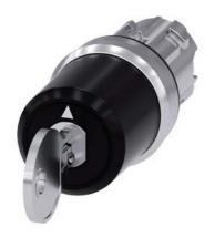
key-operated switch Siemens, 22 mm, round, metal, shiny, lock no. STGH10, with 2 keys, 3 switch positions I>O<II, momentary contact type, actuating angle 2x45°, 10:30h/12h/13:30h, key removal O, with laser labeling, lower case
