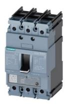
circuit breaker 3VA5 UL frame 125 breaking capacity class S 25kA @ 480 V 3-pole, line protection TM230, FTAM, In=70A overload protection Ir=70A fixed short-circuit protection Ii=5...10 x In cable connection on both sides
