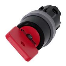
Key-operated switch O.M.R, 22 mm, round, plastic with metal front ring, lock number 73037, red, with 2 keys, 2 switch positions O-I, latching, actuating angle 90°, 10:30h/13:30h, key removal O, with laser labeling, lower case
