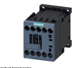
Contactor relay, 2 NC+2 NO 230 V AC, 50/60 Hz Size S00, screw terminal integrated varistor Ambient temperature -30 °C up to 70 °C, thermal rating max. 0.857 Operating range coil 0.95-1.03 US US = 230 V, Tmax 70 °C Frequency of operation 0.857 z
