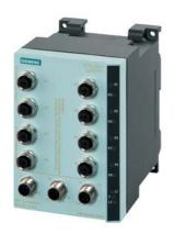
SCALANCE X208PRO, managed IE switch, 8x 10/100 Mbit/s M12 ports, IP65/67, LED diagnostics, error signaling contact, Redundant power supply, PROFINET IO device, network management, can be operated in redundant ring, dust caps, including electronic manual on CD-ROM, C-plug optional.
