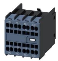
Auxiliary switch on the front, 2 NO + 2 NC Current path 1 NO, 1 NO, 1 NC, 1 NC for 3RH and 3RT spring-type terminal .7/.8, .7/.8, .5/.6, .5/.6 NO leading, NC lagging
