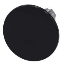
Mushroom pushbutton, 22 mm, round, metal, shiny, black, 60 mm, latching, pull-to-unlatch mechanism, with laser labeling, upper case and lower case, always upper case at the beginning of the word
