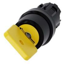
Key-operated switch O.M.R, 22 mm, round, plastic, lock number 73033, yellow, with 2 keys, 2 switch positions O-I, latching, actuating angle 90°, 10:30h/13:30h, key removal O, with laser labeling, upper case and lower case, always upper case at beginning of line
