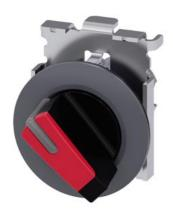
Selector switch, illuminable, 30 mm, round, Metal, matte, red, selector switch, short, front ring for flush installation, 2 switch positions O-I, latching, actuating angle  $90^\circ,\,10:30h/13:30h,$  with laser labeling, upper case and lower case, always upper case at the beginning of the word
