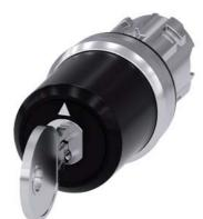
key-operated switch Siemens, 22 mm, round, metal, shiny, lock number SSG10, with 2 keys, 3 switch positions I-O-II, latching, actuating angle 2x45°, 10:30h/12h/13:30h, key removal I, with laser labeling, lower case
