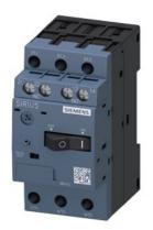
Circuit breaker size S00 for motor protection, CLASS 10 A-release 1.1...1.6 A N-release 21 A Screw terminal Standard switching capacity with transverse auxiliary switch 1 NO+1 NC
