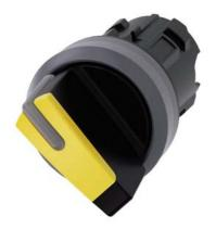
Selector switch, illuminable, 22 mm, round, plastic with metal front ring, yellow, selector switch, short, 2 switch positions O<I, momentary contact type, Actuating angle 45°, 10:30h/12h, with laser labeling, inscription or symbol Customer-specific selection with SIRIUS ACT configurator (CIN)
