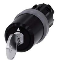
Key-operated switch BKS, 22 mm, round, plastic with metal front ring, lock number S1, with 2 keys, 3 switch positions I>O<II, momentary contact on the left, latching on the right, actuating angle 2x45°, 10:30h/12h/13:30h, key removal O, Z=50-unit packaging
