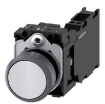
Pushbutton, 22 mm, round, plastic with metal front ring, white, pushbutton, flat, momentary contact type, with holder, 1 NO+1 NC, spring-type terminal, with laser labeling, upper case
