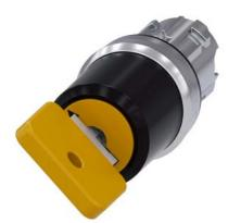
Key-operated switch O.M.R, 22 mm, round, metal, shiny, lock number 73033, yellow, with 2 keys, 2 switch positions O-I, latching, actuating angle 90°, 10:30h/13:30h, key removal I, with laser labeling, upper case and lower case, always upper case at beginning of line
