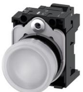
Indicator lights, 22 mm, round, Metal, shiny, white, lens, smooth, with holder, LED module with integrated LED 230 V AC, spring-type terminal, with laser labeling, upper case and lower case, always upper case at beginning of line
