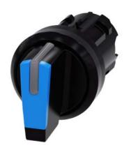
Selector switch, illuminable, 22 mm, round, plastic, blue, selector switch, short, 3 switch positions I-O<II, left latching, right momentary contact type, actuating angle  $2x45^{\circ}$ , 10:30h/12h/13:30h, with laser labeling, lower case
