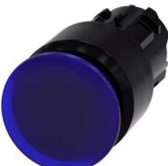
Illuminated mushroom pushbutton, 22 mm, round, plastic, blue, 30 mm, latching, pull-to-unlatch mechanism, with laser labeling, upper case
